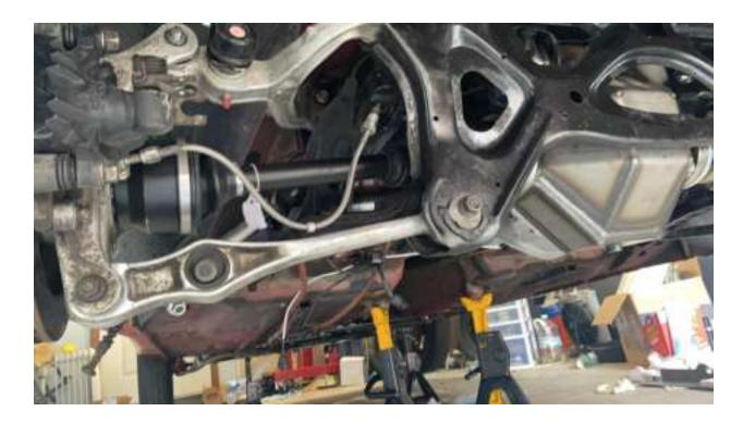
After you have the subframe back in place and your wheel hubs installed and the spindles and suspension all back in place you can install the axles into the wheel hubs and bolt on the CV's to the inner 9" stubs.
