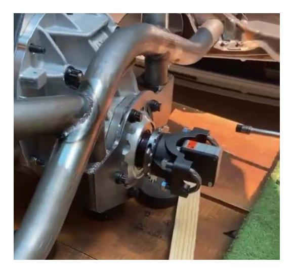
With the subframe level, now you will want to attached the x-brace to the front mount (snug only, so it can be rotated slightly for best fitment) and now use wood again to lift the front of the differential nose up so that you can get the differential to about 3 or 4 degrees of angle UPWARD.
