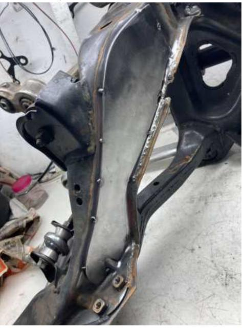
After the plates are welded in place the next step is to assemble the center section onto the rear case using the studs and nylock nuts.
