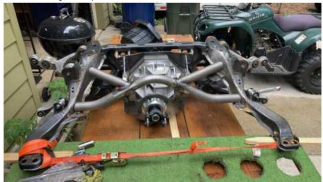
Once the rear end is fully assembled we can install it into the rear mounting holes of the OEM subframe. Leave these bolts hand tight for now as we do want to be able to rotate the differential in the subframe for the front mount positioning
