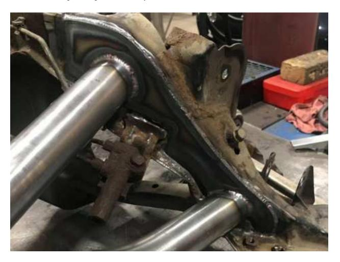
After you have the x-brace fully welded you can paint the subframe and it will all be ready for reinstallation.
