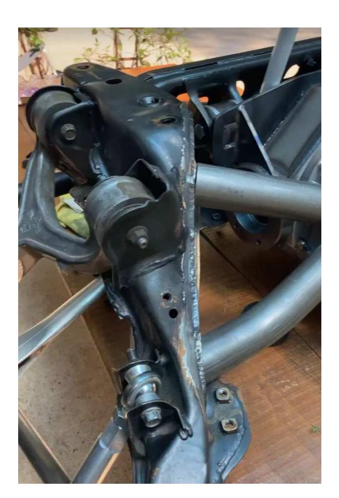
Once you have the differential yoke/input at the desired angle , you can now tack weld the x-pipe in place to the subframe reinforcement plates. Try to tack it well so it will have less tendency to move around when finish welding. You can TIG or MIG weld the x-pipe to the plates. Due to variances in the subframes you may have more gap in certain areas than others for this reason mig welding the brace may be easier.
