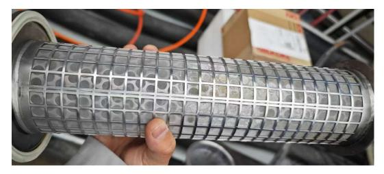
Figure 10-2 Remove the pipeline filter
