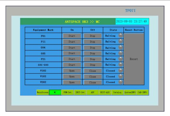
Figure 8-30 Manual control interface
