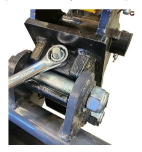
4. Loosen the head of the bolt on the bottom of the quick hitch. Doing this will raise the bottom jaw, once the jaw has moved enough off of the bottom bolt on the bucket you should be able to lift the bucket and still have it pivoting in the top jaw.
