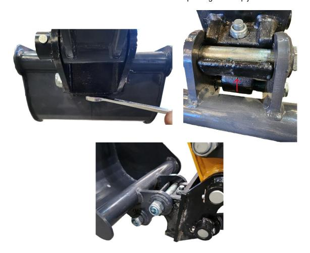
5. Lower the bucket onto the ground and reverse the steps to install a new bucket.
