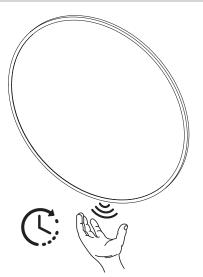
Hold your hand in front of the sensor to change the colour temperature of the light.
