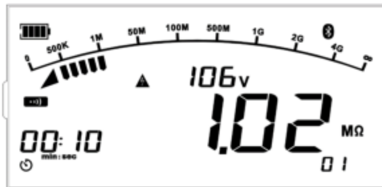
Figure 13.28 Bluetooth communication in insulation measurement mode
