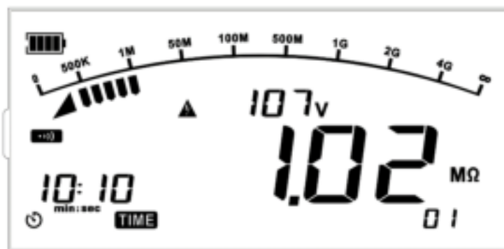
Figure 13.6 Start time-set measurement
