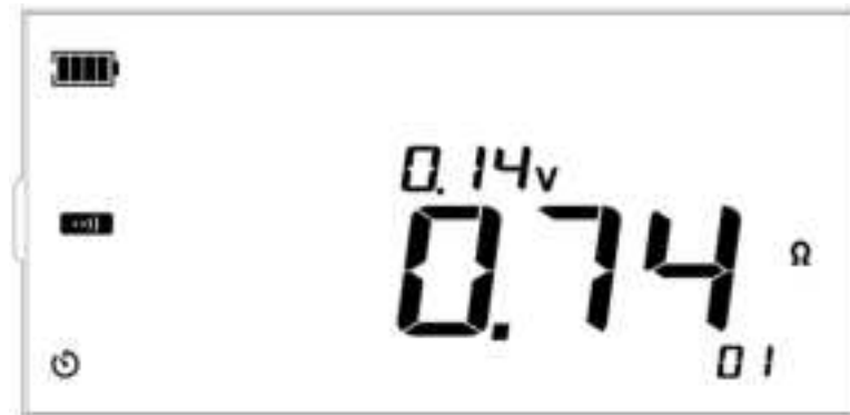
Figure 13.16 Test leads are shorted
