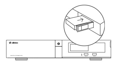
**Note:** Do not load or change the hard disk while the power is on to avoid damage of the device or hard drive data. If it is a brand-new hard disk, please format it before loading it to the device. This device supports hard disk of the following formats: EXT3, EXT4, NTFS, FAT32, EXFAT.
