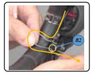
**F.** While holding the **UPPER LEVER** in place, pull the cable in a swift action.
