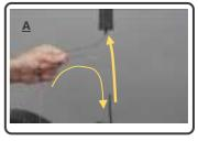
**B.** Install a barrel adjuster if not present. Reset the barrel adjuster and attach it onto the housing. Pull the cable tight to remove any slack.
