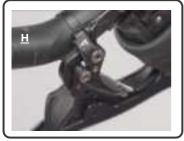
$\mbox{\bf H.}$  Tighten the pinch screw to 3Nm. Cut down the excess. Fit a cable end.
