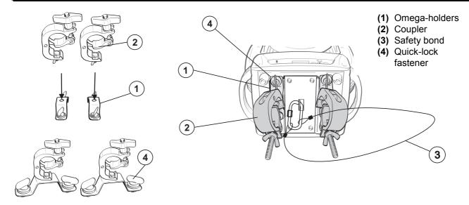
The device can be fastened via its base to a truss or similar rigging structure in any orientation without altering its operation characteristics. The device must never be fixed swinging freely in the room.
