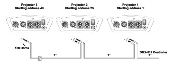
The wires must not come into contact with each other; otherwise the fixtures will not work at all, or will not work properly.
