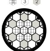
The LEDs of the device are arranged in three different segments (see graphic) and can be individually controlled with the following DMX-protocol.
