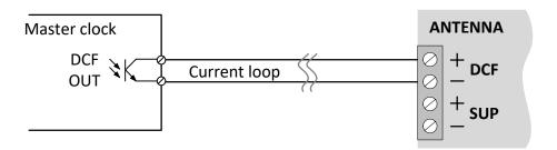
Operating threshold of the current detection: ca. 6mA. Short-circuit current: ca. 30mA.
