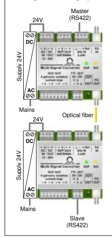
Connection of a GNSS receiver via optical fiber for the DCF synchronization of one or more systems
