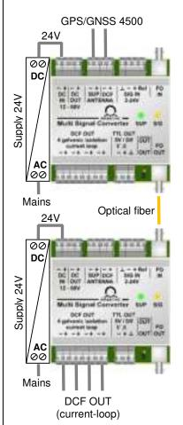
Schematic representation of the inputs and outputs
