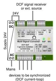
DCF-Distribution with cascading of additional distributors. Signal input: DCF 4500 (two wires) or GPS/GNSS 4500 with power supply (4 wire connection). 24V supply cascaded.
