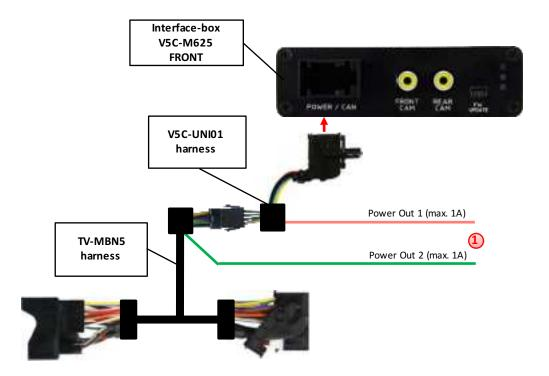
You can configure the both +12V trigger outputs separately. The pink wire is POWER OUT 1 and the green wire is POWER OUT 2.
