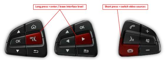
**Long press "handsfree mode OFF"** respectively **long press "right arrow" button** to choose the interface as current video source.
