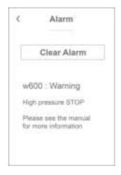
If the unit is faulty or an error occurs, there will be either a warning or an alarm. The icon will appear in the top right hand corner in the menu bar.
