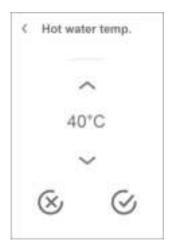
You can change the hot water temperature by using the upand-down arrows. You then confirm by pressing the confirm icon, bottom right. The main screen of the panel will then be displayed again.
