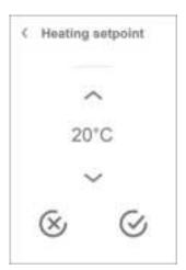
You can change the setpoint temperature for central heating by using the up-and-down arrows. You then confirm by pressing the confirm icon, bottom right. The main screen of the panel will then be displayed again.
