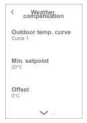
You can change the selected curve for weather compensation from this panel screen in the same way as described for the 'Central Heating' function in 'Unit Settings'.
