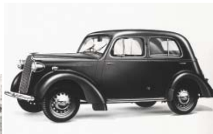
1937 – The Vauxhall 10' H-type, the first British car to have integral construction.
