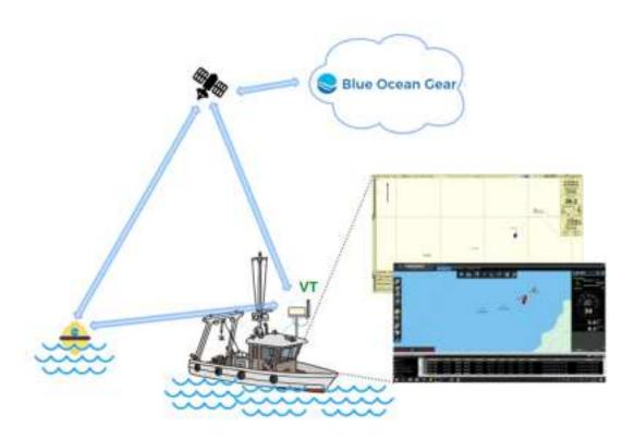
The PL makes use of both Iridium and ISM band radio links. The buoy data it receives over these links are then passed as NMEA sentences; standard to most plotters.
