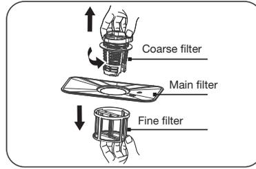
1. Hold the coarse filter and rotate it anticlockwise to unlock the filter. Lift the filter upwards and out of the dishwasher.
