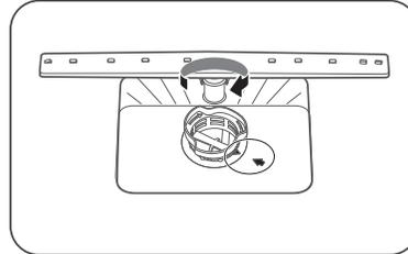
3. Larger food remnants can be cleaned by rinsing the filter under running water. For a more thorough clean, use a soft cleaning brush.
