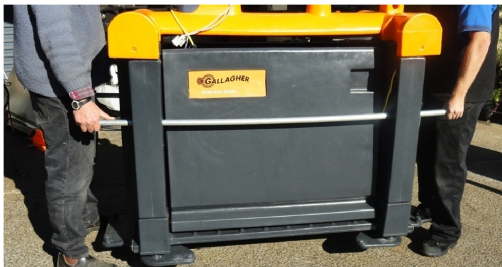
Figure 5. Lifting using the transport poles.
