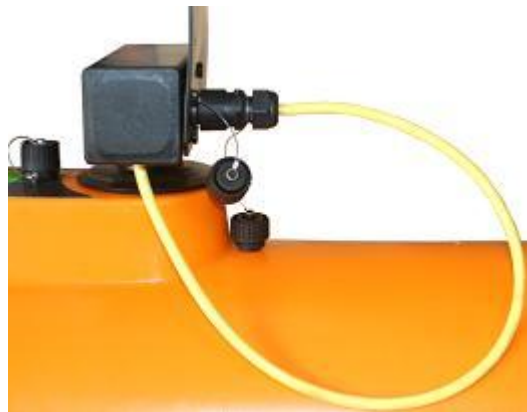
Figure 19. The loop back cable.
