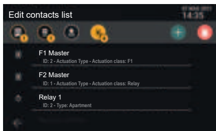
Example screen with the "Actuations" filter enabled.
