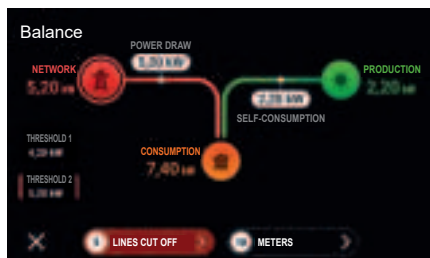
Balance graph (production and consumption [power draw] with meters and disconnected lines)
