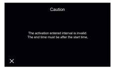
If an incorrect activation time is entered, an error message is displayed. The user is asked to set an end time later than the indicated start time. Select "Exit" to return to the screen before the time settings.
