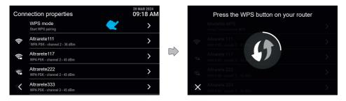
Click on the "WPS mode" row to activate this special association method; the screen displays an animation in loop. The system waits for the connection to the router, while the cancel button is used to return to the previous screen.
