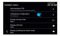
"Videophone configuration" is available, presenting information on the "ID of the indoor station (and any ID of the group it belongs to)", or, if the video entryphone is not yet configured, the wording "Not configured" will be visible.
