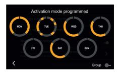
Press and hold one of the days programmed and drag onto another to copy the whole programming.
