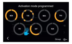
The system offers the possibility to set up to six activation time bands for every day of the week, represented as yellow sectors on a wheel representing the whole day; like the time band programming mode, with minimum start value at 0 and maximum end value at 24 (12 PM), a graphic sign marks the breaks.
