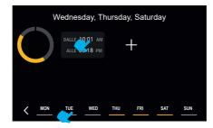
The navigation bar at the bottom of the screen shows the days, highlighting the selected ones in yellow, in this case for all the days in the group.
