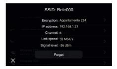
Click on the row relating to a network to access the related options: in this case, as the device is connected to a known network, only the "Forget" control is available, used to delete the information on the network connection.
