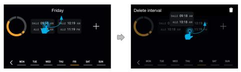
The intervals can be removed by pressing and holding the corresponding card and then dragging it upwards.
