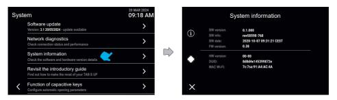
The "System information" section shows details of the software and hardware versions of the device.
