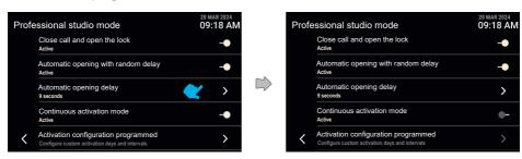
When the "Programmed activation mode" function is activated, the professional firm function is not always active. It is activated according to time slots which have been set in "Programmed activation configuration". If the programmed activation mode is deactivated, then the professional firm function is always active
