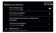
If the WiFi is active but not connected to any network or connected physically but without an IP address, the connection to mobile devices will not be available and will be shown as inaccessible.
