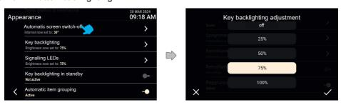
Click on the "Key backlighting" row to change the backlighting intensity and view a preview of the effect applied to the device
