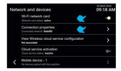
The "Network and devices" section allows you to control all the video entryphone connectivity parameters; for the first item, it is possible to activate Wi-Fi.
