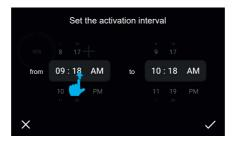
Click on "Add" to view a pop-up to select the start and end time in tumbler mode; the band start time is set with the current value and the end time with the current value + 1 hour.
