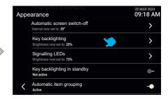
Click on the "Signalling LEDs" button to change the brightness of the LEDs in the indicated options. Click on the cancel button to return to the previous screen.
