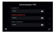
If the new PIN entered is the same as the current PIN, the screen displays an error message; change the new PIN entered and proceed.
