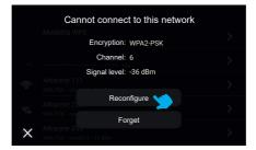
If it is not possible to connect to the network, the only information available is the coding, the channel and the signal level. The available actions are: "Reconfigure" or "Forget". Selecting reconnect to the network, the password setting screen appears.
