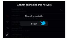
If it is impossible to connect to the selected network due to lack of signal, the only control available is "Forget".
