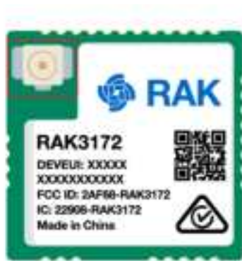
Figure 3: IPEX Connector of RAK3172 for LoRa Antenna
