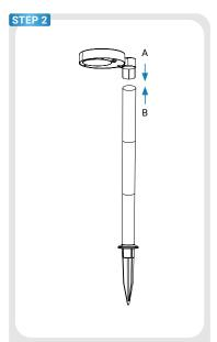
a. Connect the light pole (B) to the light (A).
