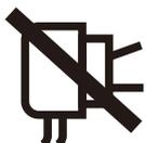
The power supply unit shall not be used, if pins of the plug part are damaged.
