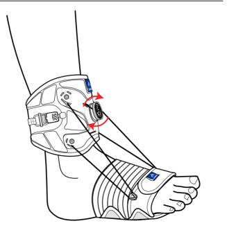
Tighten cords by turning dial clockwise to raise foot to desired position.
