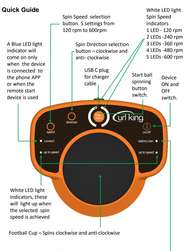
This red indicator will flash quickly when the device needs charging.  $^{\mathsf{T}}$  The red light will flash slowly when the Curl King $^{\mathsf{TM}}$  is being charged. Once the device is fully charged the red light will be on constantly.
