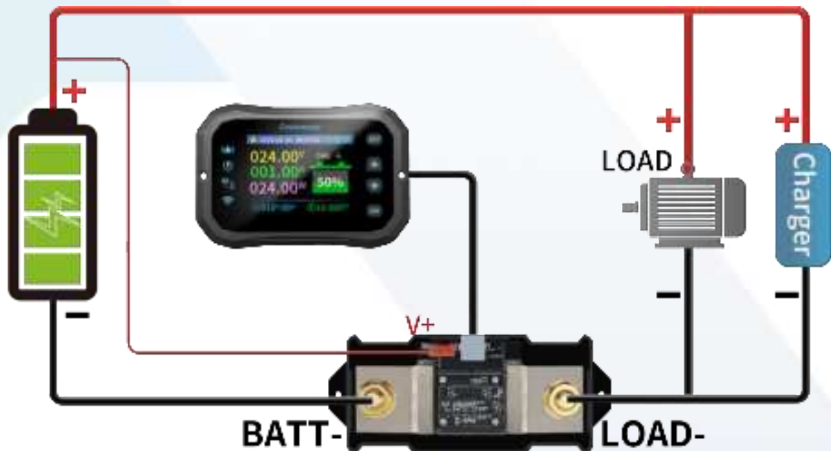
Figure 2-3-2: 100A/400A/600A Sampler Wiring Diagram (illustrated with 400A)
