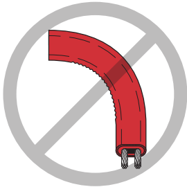
Figure 7: Bending the SC heating cable
