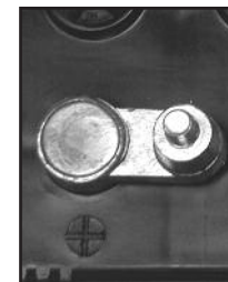
POSITIVE POST HAS LARGER DIAMETER
