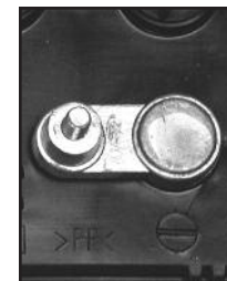
NEGATIVE POST HAS SMALLER DIAMETER
