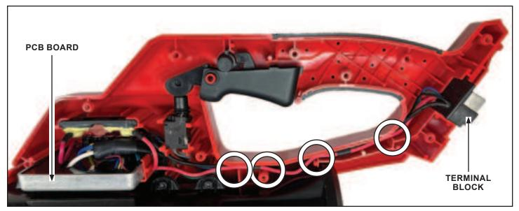
4) When routing the wires from the Terminal Block to the PCB Board, please make sure the wires fit securely inside the traps and between the ribs without pinching the wires.
