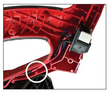
3) Make sure the RED wire is on top of the other wires through the slim grooves. The BLACK wire (thick one) should be in the middle and the remaining wires should be below them.
