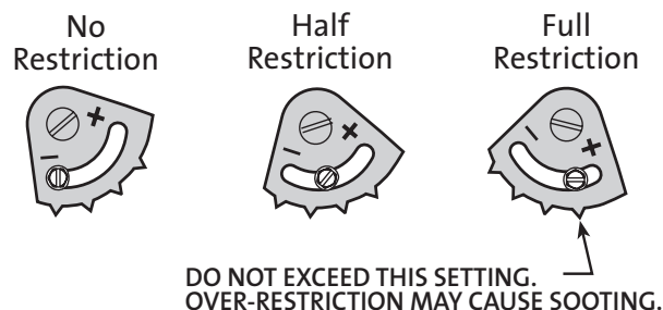
Figure 15. Exhaust Restrictor settings
