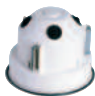
Figure 3.1: Ceiling mount back box The ceiling-mount back box (refer to figure) is made of white polypropylene. It has four cable bushings with tight-closing rubbers lips of polyflam that are suitable for cable diameters up to 1.4 cm. When used with a base, approx. 30 cm of cable length can be accommodated in the upper area of the ceiling-mount back box.
