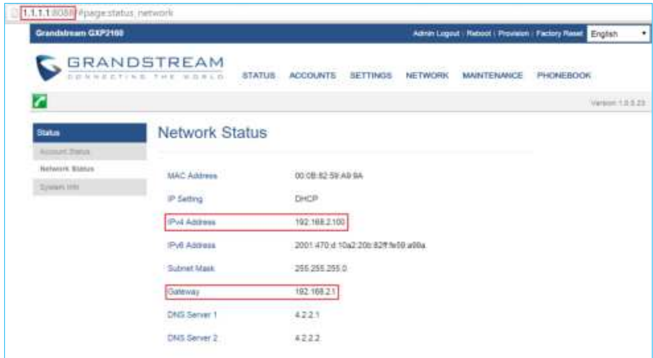
Figure 26: GXP2160 Web Access using UCM6302A Port Forwarding
