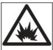
Risk of Explosion
