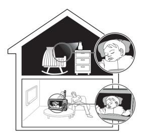
The baby unit has infrared LEDs that allow you to see your baby clearly at night or in a dark room. When the baby unit being viewed detects low light levels, the infrared LEDs are switched on automatically. The images from the baby unit are in black and white, and 2 appears on the parent unit screen.
