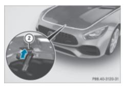
Reach into the gap, pull bonnet catch handle ② up and lift the bonnet.
