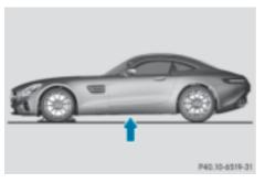
The jacking point is in the centre between the front and rear wheel arches (arrow).
