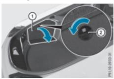
The vehicle tool kit is located in the left-hand stowage compartment behind service flap ① in the luggage compartment.
