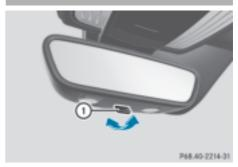
► Anti-dazzle mode: pivot anti-dazzle switch (1) forwards or back.
