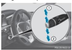
You can use the cruise control lever to limit the speed to any speed above 30 km/h while the engine is running.
