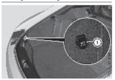
The battery may drain if the vehicle is left stationary for long periods. In this case, Mercedes-Benz recommends attaching the trickle charger to the 12 V socket in the luggage compartment.
