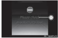
Warning message ① is displayed in the instrument cluster if Traffic Sign Assist detects that you are passing a "no entry" sign and you are driving in the wrong direction. You will then also hear a warning tone. You should immediately check your direction of travel in order to avoid danger to yourself and other road users.
