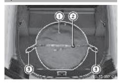
The collapsible emergency spare wheel is secured in emergency spare wheel bag ① in the luggage compartment.
