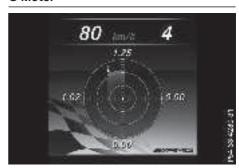
The G-Meter shows you the forces that are exerted on the driver during the journey, both laterally and in the direction of travel.
