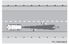
Distance Pilot DISTRONIC has not yet detected the vehicle in front on the edge of the carriageway because of its narrow width. The distance to the vehicle in front will be too short.
