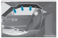
Windowbags ① are integrated in the side of the roof frame above the doors.
