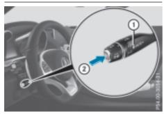
Check whether LIM indicator lamp ① is off. If it is off, Distance Pilot DISTRONIC is already selected. If it is not, press the cruise control lever in the direction of arrow (2).
