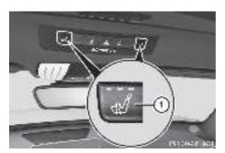
The three red indicator lamps in the button indicate the heating level you have selected.
