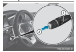
► Check whether LIM indicator lamp ① is off. If it is off, cruise control is already selected. If it is not, press the cruise control lever in the direction of arrow ②.
