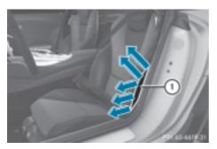
Sidebags ① deploy next to the outer bolster of the seat backrest.
