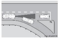
Distance Pilot DISTRONIC does not brake for obstacles or stationary vehicles. If, for example, the detected vehicle turns a corner and an obstacle or stationary vehicle is revealed, Distance Pilot DISTRONIC will not brake for them.
