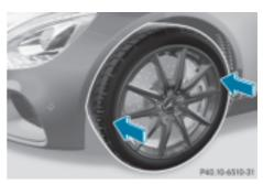
► Slide the wheel to be mounted onto the centring pin and push it on.
