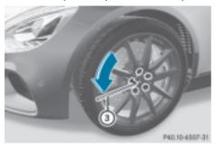
Using wheel wrench (3), loosen the bolts on the wheel you wish to change by about one full turn. Do not unscrew the bolts completely.
