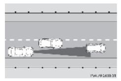
Distance Pilot DISTRONIC may not detect vehicles which are not driving in the middle of their lane. The distance to the vehicle in front will be too short.
