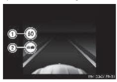
A maximum permissible speed of 60 km/h (60 mph) ① and an overtaking restriction ② apply.
