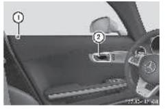
▶ Pull door handle ②. If the door is locked, locking knob (1) pops up. The door is unlocked and opens.
