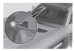
Lane Keeping Assist monitors the area in front of your vehicle by means of multifunction camera (1) attached at the top of the windscreen. Lane Keeping Assist detects lane markings on the road and can warn you before you leave your lane unintentionally.
