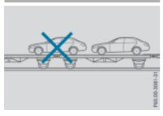
When the vehicle is loaded for transport, the front and rear axles must be stationary and on the same transportation vehicle. Positioning over the connection point of the transport vehicle is not permitted. The drive train may otherwise be damaged.
