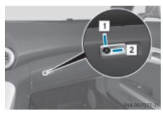
The glove compartment can be locked and unlocked using the emergency key element.
