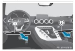
Driver's kneebag ① deploys underneath the steering column and front-passenger kneebag ② underneath the glove compartment. The driver's and front-passenger kneebags are triggered together with the front airbags.
