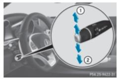
➤ To adjust the set speed in 10 km/h increments: briefly press the cruise control lever up ① beyond the pressure point for a higher speed, or down ② for a lower speed.
