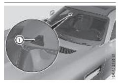
Traffic Sign Assist displays the maximum speed permitted and overtaking restrictions to the driver in the instrument cluster. Driving onto a section of road in the wrong direction triggers a warning. Traffic Sign Assist detects traffic signs with multifunction camera ① attached at the top of the windscreen. The data and general traffic regulations stored in the navigation system are also used to determine the current speed limit.
