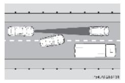
Distance Pilot DISTRONIC has not detected the vehicle cutting in yet. The distance to this vehicle will be too short.
