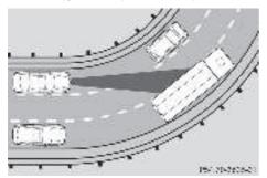
Distance Pilot DISTRONIC can detect vehicles when cornering is limited. Your vehicle may brake unexpectedly or late.
