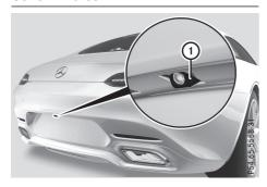
Reversing camera ① is located in the rear bumper, underneath the tailgate.
