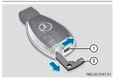
▶ Push release catch ① in the direction of the arrow and, at the same time, remove emergency key element ② from the key.
