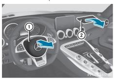
Driver's airbag ① deploys in front of the steering wheel. Front-passenger front airbag ② deploys in front of and above the glove compartment.
