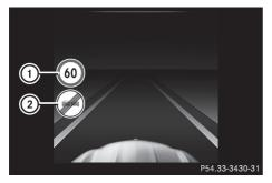
A maximum permitted speed of 60 km/h (60 mph) ① applies. The overtaking restriction no longer applies ②. The traffic sign indicating the end of an overtaking restriction is displayed for five seconds.
