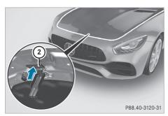
Reach into the gap, pull bonnet catch handle (2) up and lift the bonnet.
