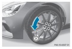
Using wheel wrench (3), loosen the bolts on the wheel you wish to change by about one full turn. Do not unscrew the bolts completely.
