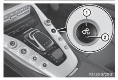
▶ Press M button ①. Indicator lamp ② lights up. The letter M appears in the multifunction display. Manual mode M is activated.
