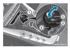
You can place insert (4) into the cup holder on the left-hand or right-hand side.
