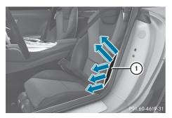
Sidebags ① deploy next to the outer bolster of the seat backrest.
