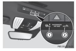
PASSENGER AIR BAG ON indicator lamp ① and PASSENGER AIR BAG OFF indicator lamp ② are part of the automatic deactivation system of the front-passenger front airbag.
