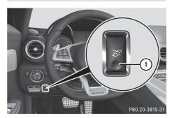
You can unlock the tailgate from the driver's seat when the vehicle is stationary and unlocked.
