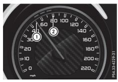
If Distance Pilot DISTRONIC detects a vehicle in front, segments between speed of the vehicle in front (1) and stored speed (2) light up.
