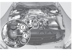
Example: checking the coolant level
