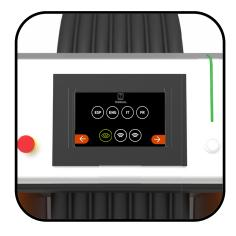
To link a controller, press the icon (🔊) on the left of the screen. The LED strip will turn blue and flash for 20 seconds.
