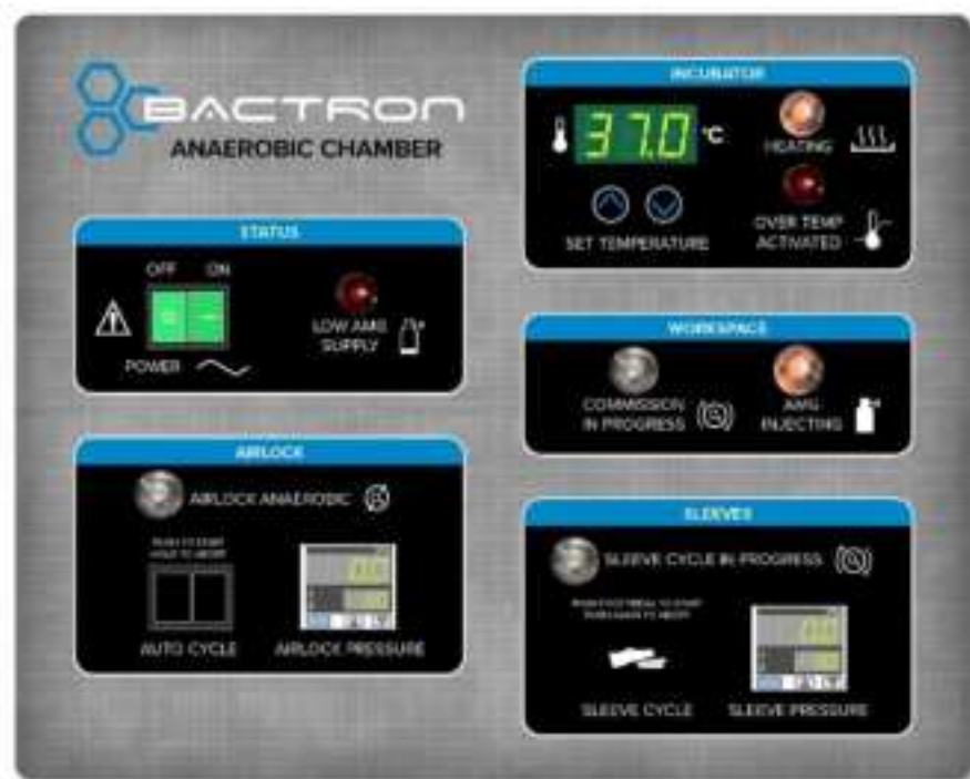
Figure 5: Main Control Panel
