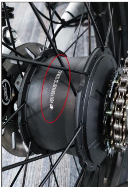
The motor serial number is located on the face of the motor.
