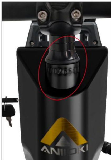
The serial number of the bike frame below the bottom bracket.
