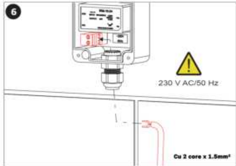
Pass mains (230V) power supply into mounting box via grommet and terminate accordingly
