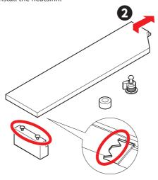
3. If you install 2260 SSD, install the supplied M.2 standoff in 2260 hole. Skip this step if you install 2280 SSD.
