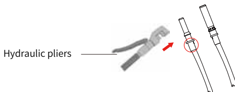
Pic 5.4 Crimp the contact pin to the wire
