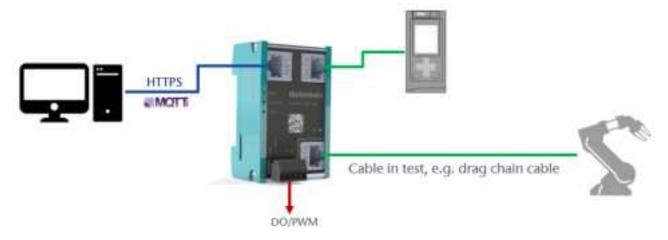
For integration into IIoT structures, the monitored cable status can also be sent via MQTT by the Cable Guard.
