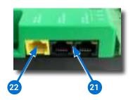
**NOTE:** The Ethernet patch cable should be T568B Category 5 (or better) and a maximum of 328 feet (100 meters) between devices
