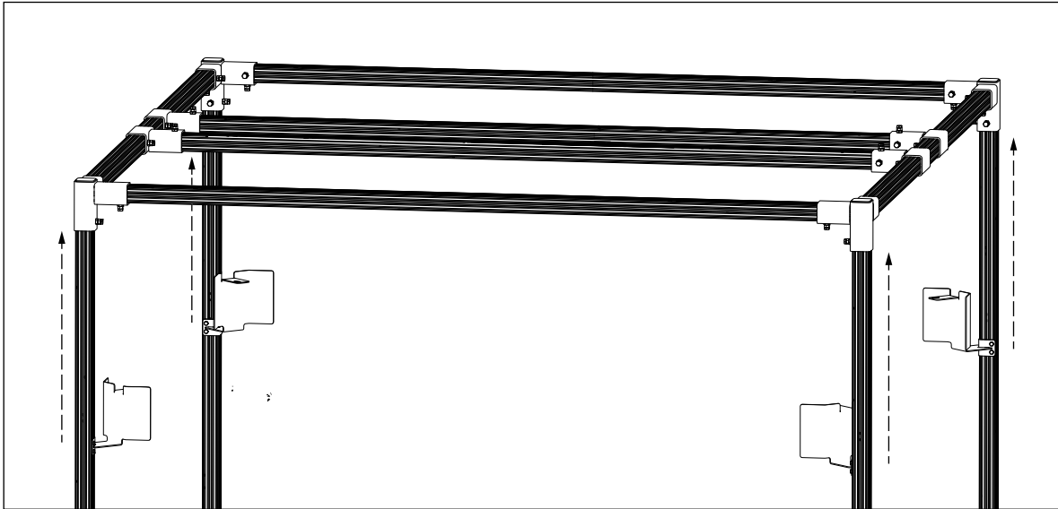
Figure 3-14. Remote IFM Sensor Assembly Attachment
