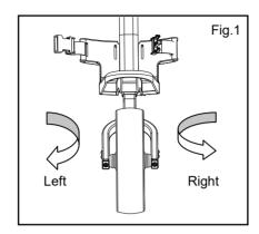
2.If the cart veers to the left, face the front wheel of the cart and use the Allen wrench provided to screw the right bolt counterclockwise or the left bolt clockwise until the front wheel is centered between the front fork.(Fig.2)
