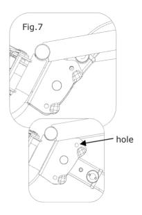
Press the red button to release the front wheel, then fold until the pin is inserted into the hole as shown in Fig.6 and Fig.7
