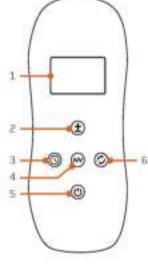
Made Button: Press to toggle through the three modes: red mode (660nm), near-infrared mode (650nm), and red + near-infrared mode (660+650nm).
