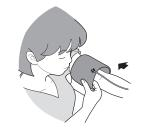
The bottom edge of the arm cuff should be 1 to 2 cm above the elbow. Air tube is on the inside of your arm and aligned with your middle finger.
