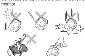
Use a soft and dry cloth, or a soft and moistened cloth and neutral soap to clean on the monitor and the arm cuff. Changes or modification not approved by the manufacturer will void the user warranty. Do not disassemble or attempt to repair the monitor or components. Consult your local OMRON representative.
