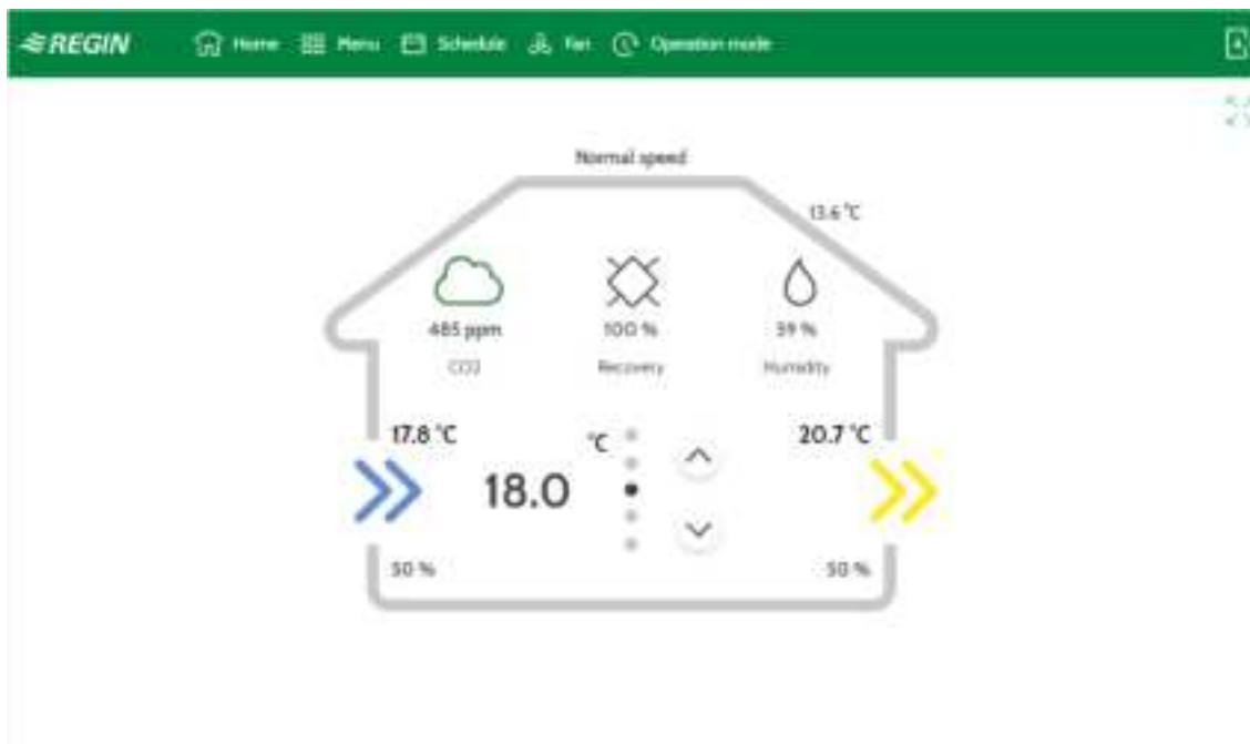
Figure 3-4 Start screen, web interface
