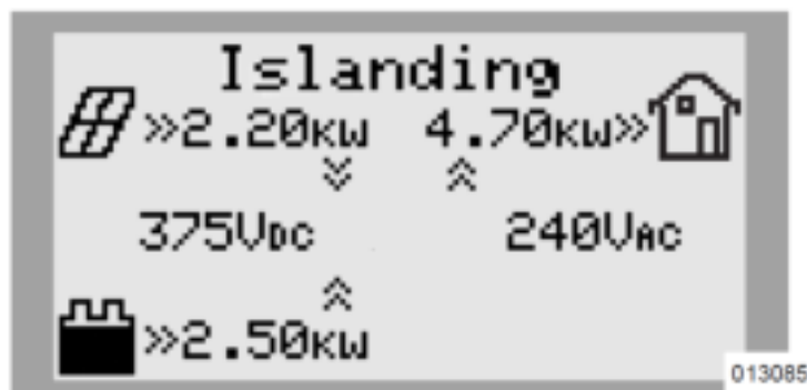
Figure 4. Island Mode with the Generator Inhibited.
