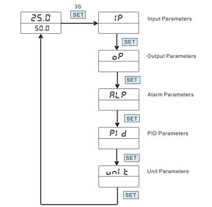
1) Press SET button for 3 seconds to enter into main menu, Output Parameters, Alarm Parameters, PID Parameters and Unit Parameters can be selected. Then press shift button to enter into the submenu if need to change the settings.
