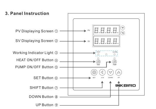
1 PV Displaying Screen: Display the measuring value or the setting parameters. 2 SV Displaying Screen: Display setting value or the set parameters readout.
