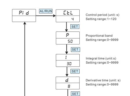
1) Ctl: Control period, setting range 0.5-120 seconds (0=0.5second), the controlling accuracy will be higher if set Ctl within 4 seconds when in SSR control output, and normally set Ctl to 20 seconds when in relay control output. The time of Ctl can be shortened if there is not the satisfaction temperature controlling required. But based on
