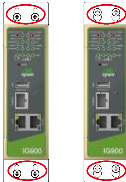
Figure 3-4 Wall mounted installation diagram
